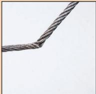
Steel wire rope bent → See the repair instructions 'CHOCKS'
