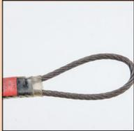
Flash rust/corrosion visible → See the repair instructions 'CHOCKS'
