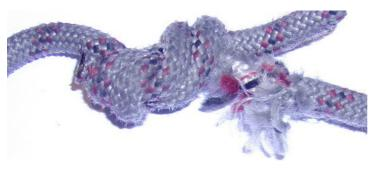
Fig.1: fibre breaks
