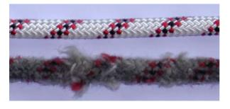
Fig. 2: Severe rope wear, wear with rope thickening
