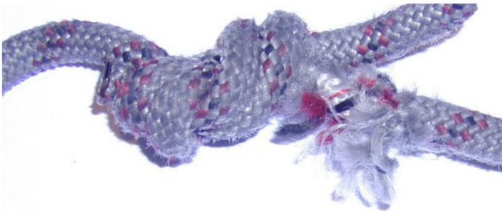
Fig.1: fibre breaks
